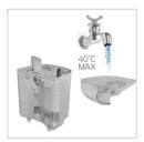
Rinse the dirty water tank and lid under water (max 40°C) to remove dirt/debris
