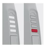
When the machine is in use the battery level indicator lights will illuminate indicating how much charge is remaining. When less than 20% charge is remaining the bottom light will flash red indicating the battery is running low and charging is required.
