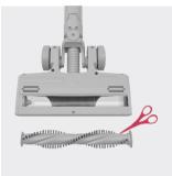
To remove any threads or hair, slide the blade of a pair of scissors into the groove on the brushbar and cut along the groove.
