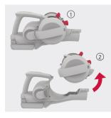
Squeeze the latch on the dirt container to release.
